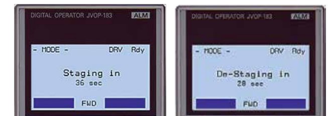
Typical multiplex keypad messages
